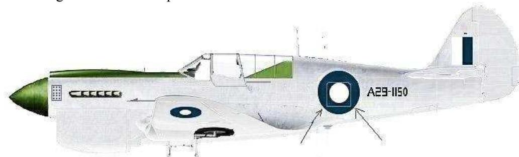
*The P-40N-40 Tac/R Prototype when completed in 1945. Notice the wider entry door on the fuselage roundel. GRB*
