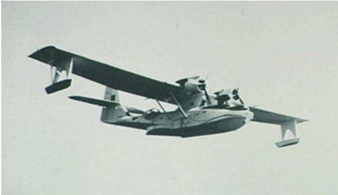
A trans-pacific RAAF PB2B-2 arriving in Australia at Rathmines near Sydney NSW in July 1945 still with the original engine de-icer heater exchangers, but without De-icing boots. AWM
