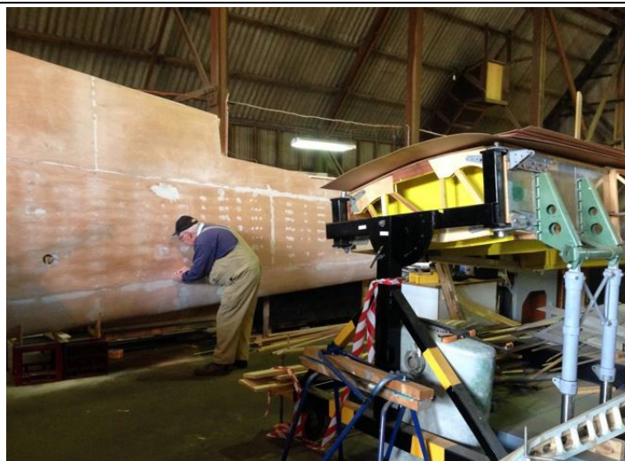
Putting the finishing touches on the Oxford's left wing – the centre section is seen in its jig on the right side of the frame
