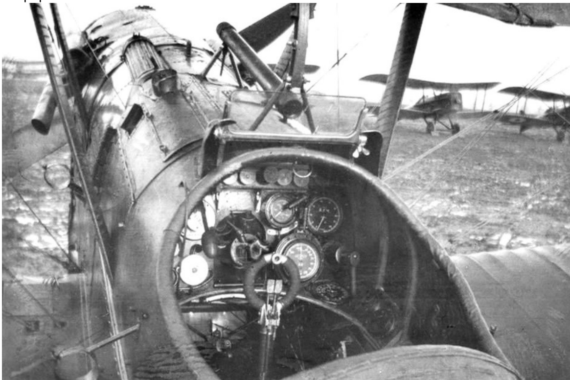
Cockpit of the S.E.5a, showing the Aldis sight and Vickers gun [IWM Q67871]
