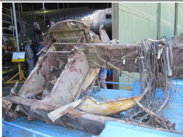
The wing centre section from a wrecked Oxford seen soon after it had arrived via donation from South Australia. This item provided many useful original (small) parts, templates and details for the project.
