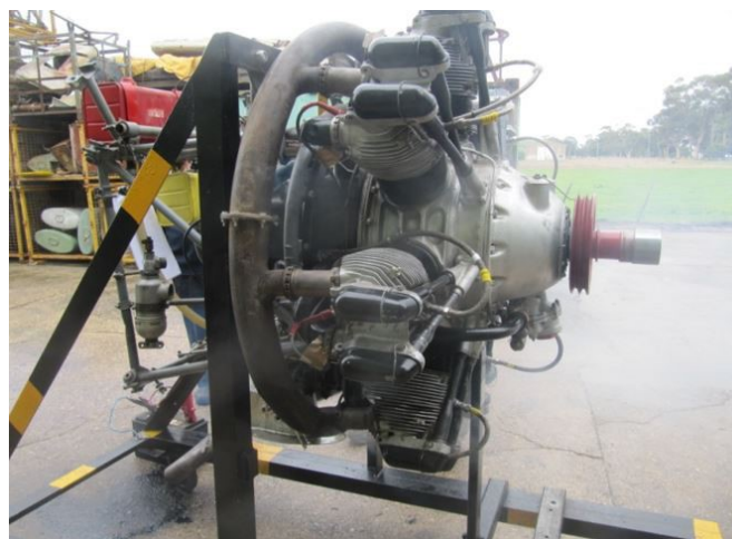
One of the project's two Armstrong-Siddeley Cheetah engines has been restored to running condition
