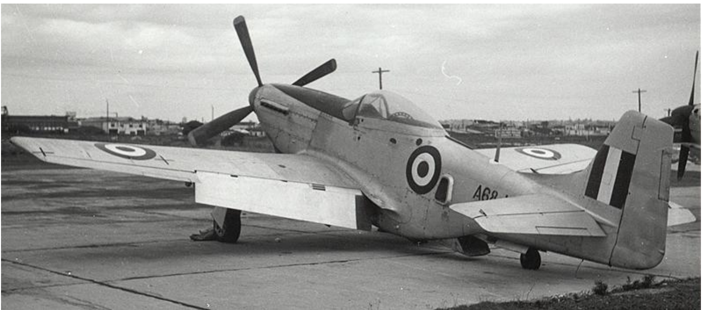
Notice camera aiming Crosses per A68-187 'S port wing. These are lined up with similar ones on canopy for alignment
