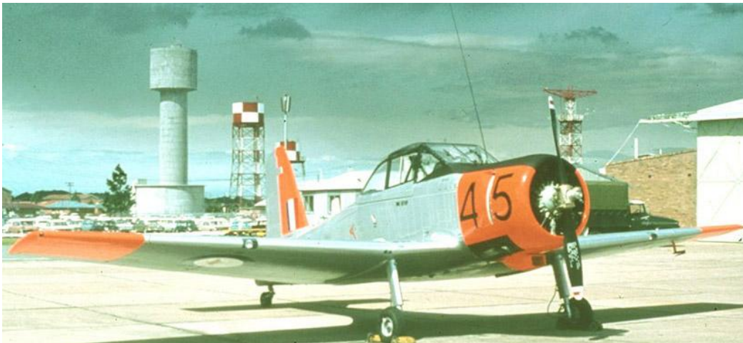
A85-445 – one of the first FAC Winjeels – at 2(F)OCU Williamtown in 1968, with the long whip antenna
