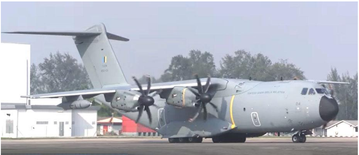
The Malaysian A-400M Atlas M54-04 is interesting, with AAR pods under the wings and its refueling probe
