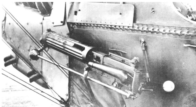
The forward-firing 0.303" Vickers machine gun used a hydraulically operated Constantinesco interrupter gear 122
