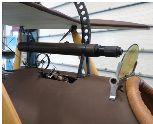
The Aldis (here on an S.E.5a) was a telescopic sight, shown also with a fixed ring-and-bead sight
