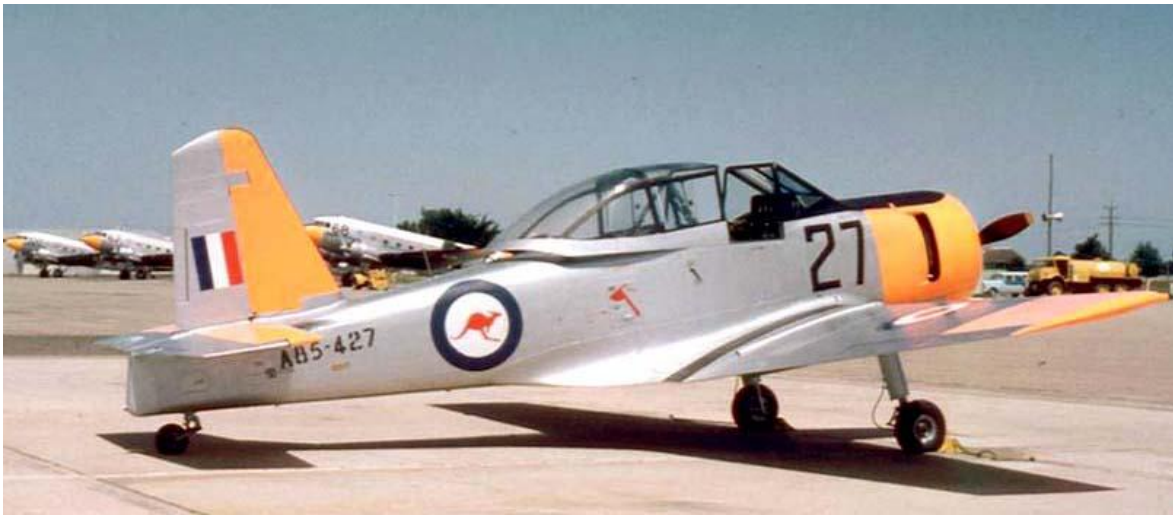
A85-427 CFS East Sale 1961 – large 33" roundel, 18"x15" flash on the rudder, nose number not on dayglo cowl This style of markings was maintained until at least late 1963
