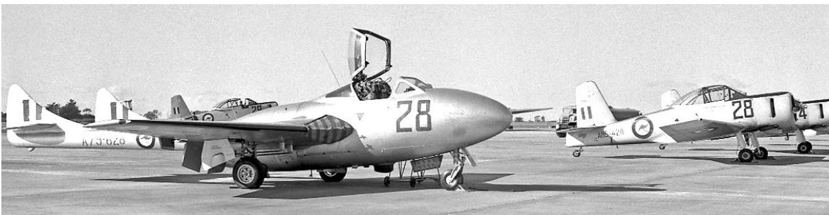
A85-428 in MAY 1961 – 'daygloed' the previous month, the large nose numbers behind the dayglo cowl and the same font/size as CFS Vampires (24"x12"), serial number (like A85-427 above) is stencilled, tail flash on rudder
