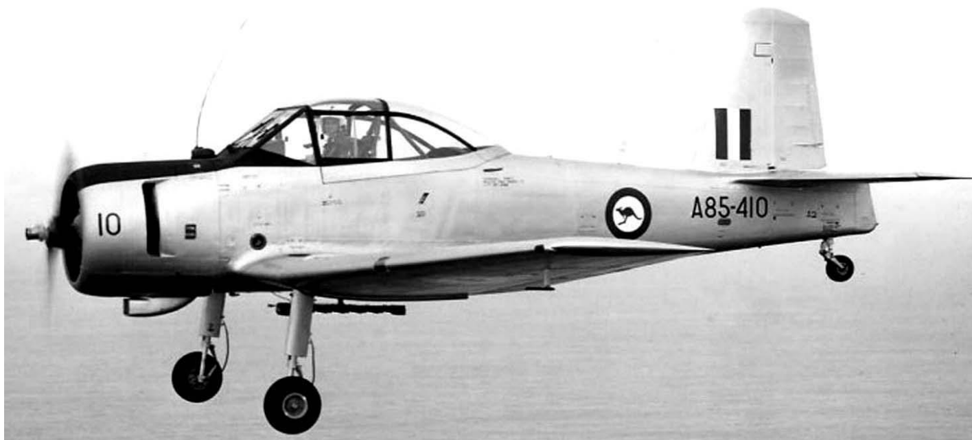
A85-410 c1971 (above) FAC-modified with the FM whip aerial and centreline smoke-grenade dispenser; and in 1974 (below), camouflaged and more clearly showing the dorsal UHF aerial – A85-410 is now on display at the Queensland Air Museum, Caloundra
