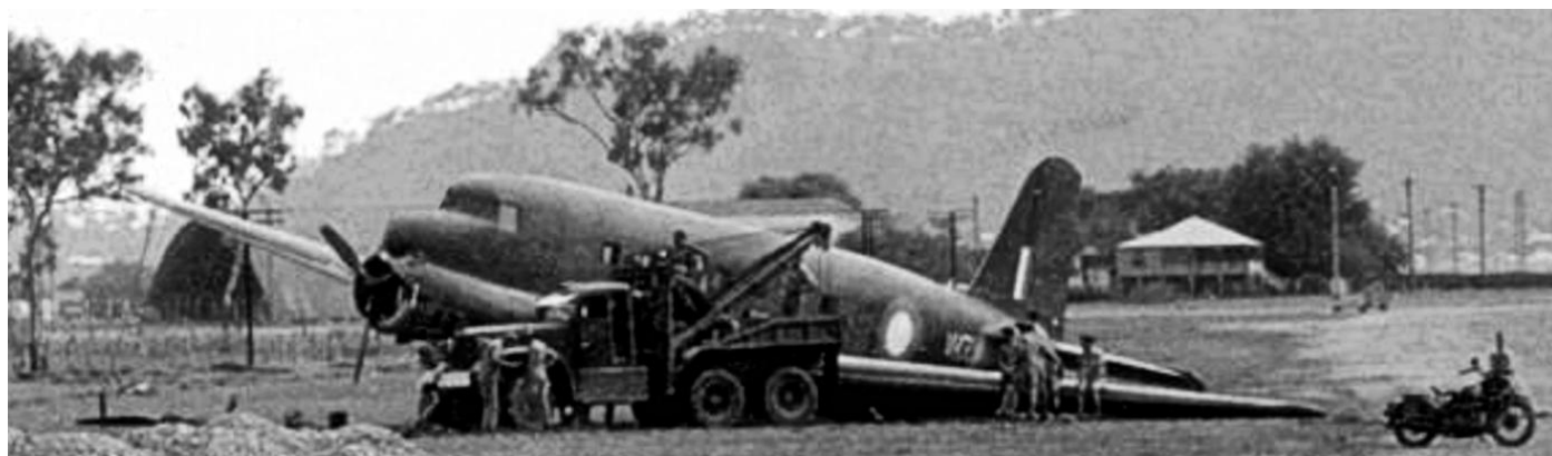
A30-6, at rest after suffering an undercarriage collapse at Townsville in September 1942. Source: RAAFWA
