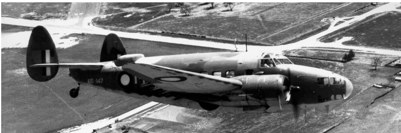
A16-147 modified to C-63 standard, serving as “M” with No 4 Communication Unit in November 1943. Bath tub refitted, in lieu of Bristol Turret. Later coded as PK-K, it would serve in No 38 Squadron RAAF.
