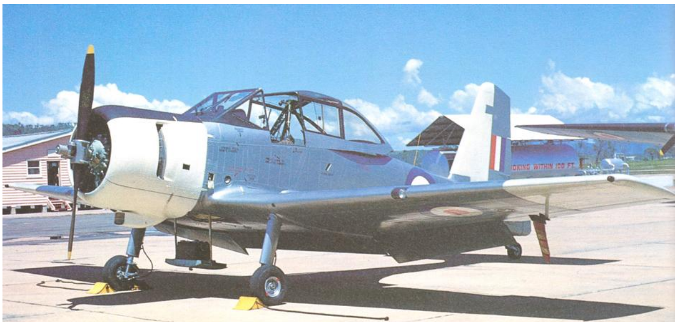
The dayglo process – a Winjeel prepared with white primer prior to application of coats of dayglo Blaze Orange
