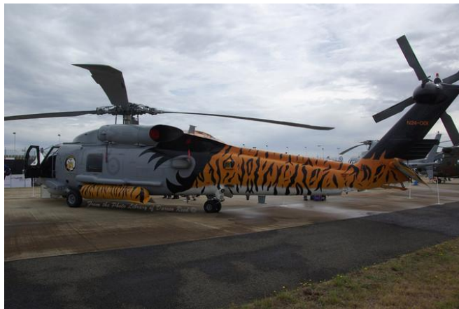
Sikorsky Seahawk "Tiger" S70B-2 N24-001 and Some tell tails signs of rear boom exchanges, N24-015 now with the recycled tail of N24-002 in place. Photos: Darren Reed and Daniel Leahy respectively
