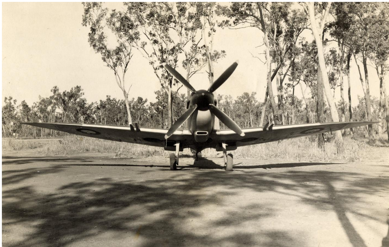
A58-482 TS-V as fitted with 4 x 20mm Cannon Dec 1944
